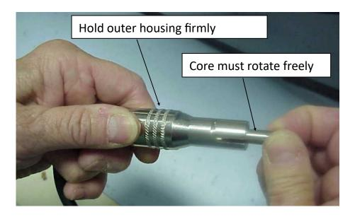
4.18 Remove outer housing. Use 5/8" and 1/2" open end wrenches to loosen the compression sleeve a little, but it must not be loose. It should remain snug. Re-assemble and re-test for free rotation. Also, make sure the cord is firmly strain relieved. If strain relief is lost, cable is
