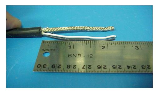
4.3 Cut center conductor to about 1.25" (3.2 cm) length shown.
