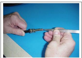
4.23 Push grommet into connector using pin depth gauge.
