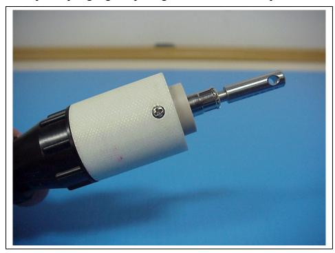
4.29 Install SHV10 feedthru tooling to fully eat the grommet.
