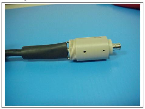
4.25 Screw cable clamp onto the housing. Tighten both screws. Make sure cable is secure in clamp. If loose, clamp may be installed upside down.
