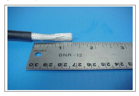
4.4 Remove fiberglass sheath to expose two safeconn wires (black and white), and shielded center conductor. Remove clear plastic wrap from braided shield.
